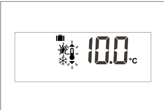
If when moving one of the set points we come to less than one degree from the following set point, it will be "dragged" so as to avoid the unsuitability of the set points. When this happens, the thermostat will flash the icon of the occupation mode of this set point being dragged.
