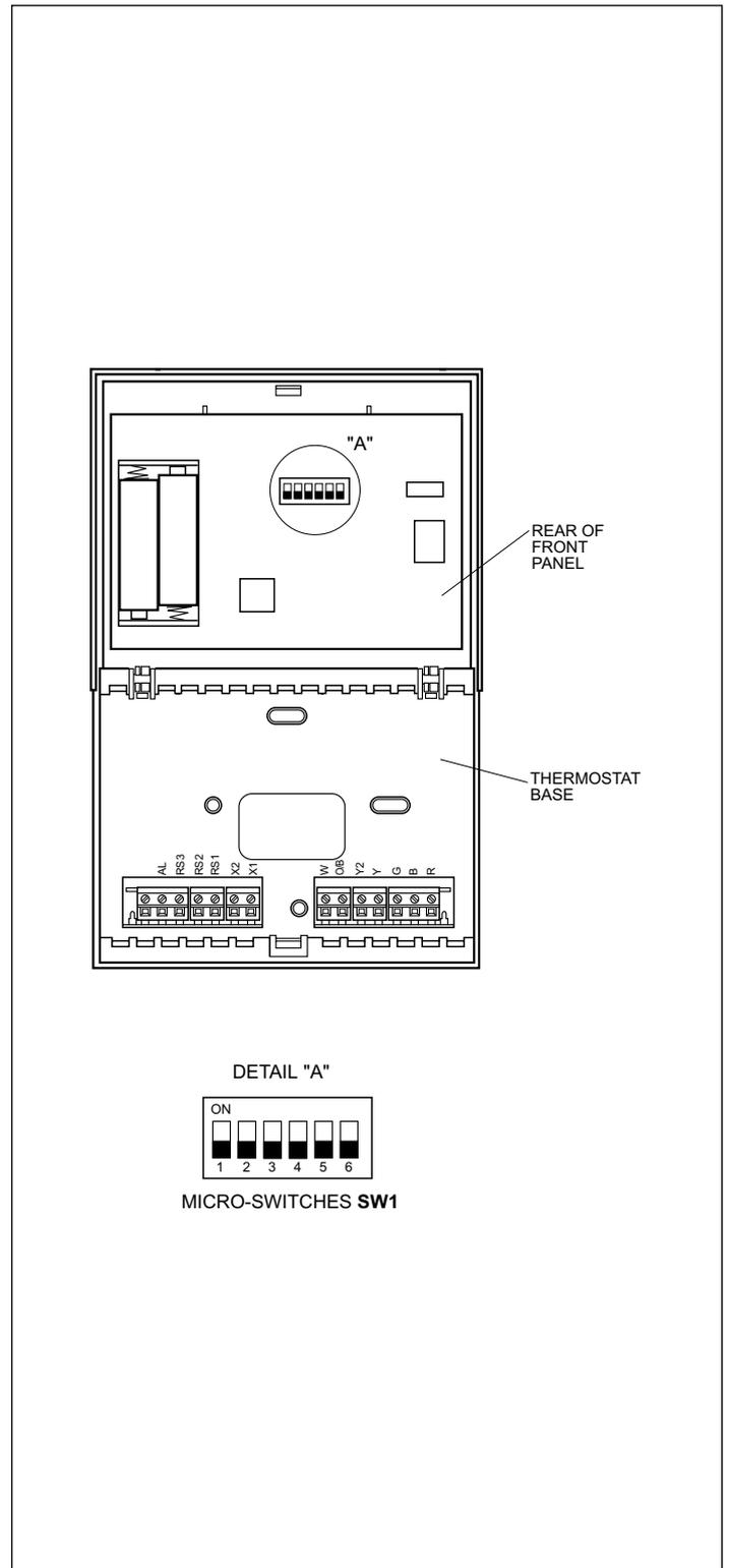
Micro-switch SW1 allow the configuration of the following parameters:
