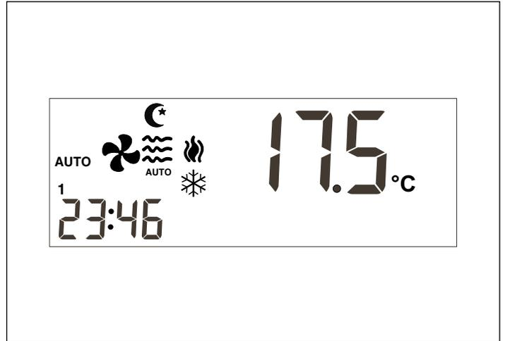
A demand is generated when the room temperature is above the cooling set point or below the heating set point. In automatic mode, room temperature is kept at a value between these two programmed set points.
