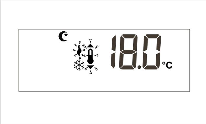
If when moving one of the set points we come to less than one degree from the following set point, it will be "dragged" so as to avoid the unsuitability of the set points. When this happens, the thermostat will flash the icon of the occupation mode of this set point being dragged.
