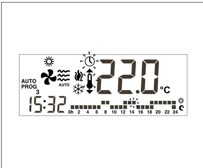
with the mode programmed in the time schedule profile, the icon of the selected mode will be displayed flashing, along with the icon, also flashing, indicating this is temporary. When a status is changed in the time schedule profile, the occupation status will go back to the status programmed in the profile (without flashing), and the icon will disappear.
