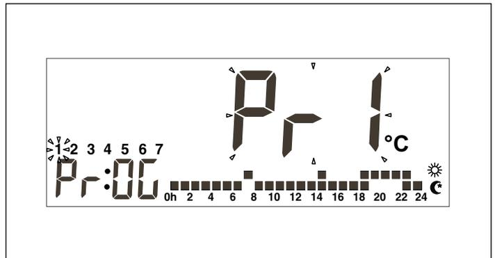
If the communication profiles are not empty, which means they are not on 24-hour stand-by, or a profile above the first six (three predefined and three user-programmable) has been selected by means of communication with the PC, profiles P7 to P12 can be selected. Should this not be the case, these profiles can neither be selected nor are displayed on screen.
