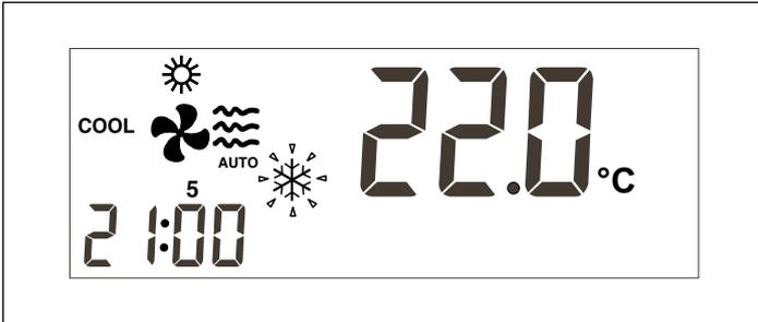
A demand is generated when the room temperature is above the programmed set point. Set point is understood as the temperature we want in the room. How to program and change set points will be described further below.
